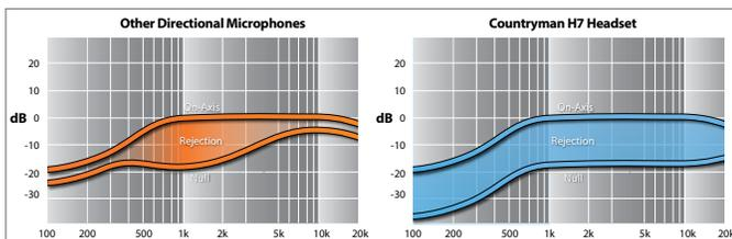
**Full-Range Directionality:** Many directional microphones are not very directional at low and high frequencies, resulting in off-axis coloration, more ambient noise, and opportunities for feedback. The H7 Headset has an extremely controlled polar pattern across frequencies for natural sound and consistent performance in any environment.
