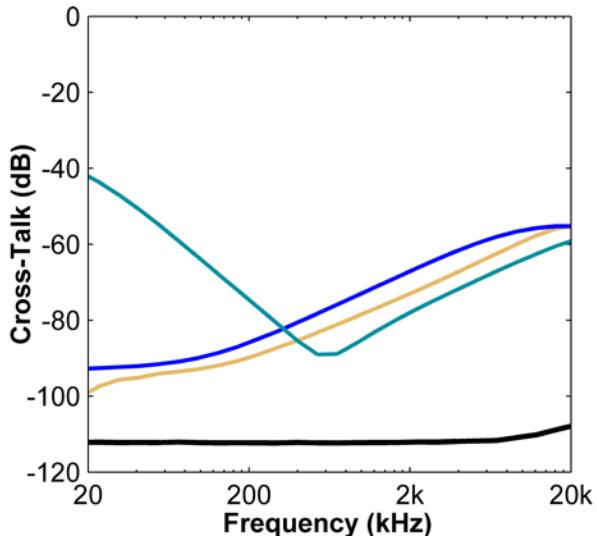
Cross-talk rejection vs. frequency for the Type 10S (black) and three of the most popular competitor stereo DIs. The Type 10S outperforms its competition by 20-60 dB for the full audio range.
