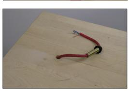
6. Feed the wire through the hole and the lower half of the A4CDM
