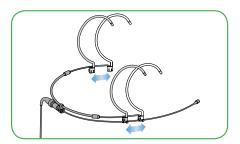
Adjust the earwires for your head size. The headset should feel snug without pinching. If the H6 feels loose on the head, slide the earwires back to tighten the fit.
