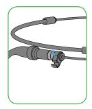
Unclip the boom from the clips at the back of the headset.
