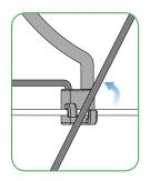
Tip the boom to remove it from the hooks on the earwire.
